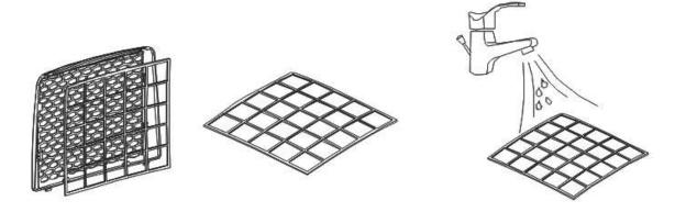
**Assemble the filter:** Insert the filter back to machine slowly after washing.
