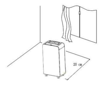
Install the unit one the flat floor and keep the room ventilated. Leave at least 20cm spacing around the unit before connecting the hose.
